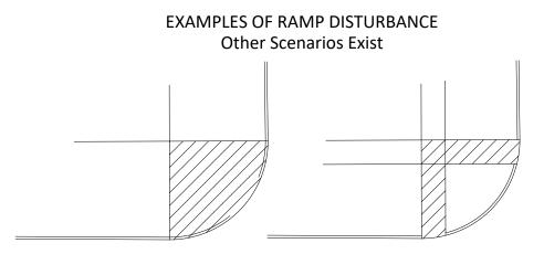
If hatched area is disturbed entire ramp and landing is to be brought to current ADA (PROWAG) standards. Additional walk and curb & gutter is to be removed and replaced as needed to bring ramp to standard.
